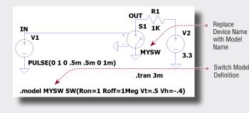
One classic application of voltage-controlled switches is simulating open-circuit and short-circuit conditions. In the example shown, two switches simulate a short- and open-circuit condition on an LED string.
